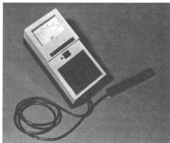
Fig.4 The device with logarithmical scale for the measurement of intensity values in the limits of 10^{-4} ÷ 10 mW/cm 2 from the range of wavelengths 280÷400 nm. The supplying is 4.5 V
