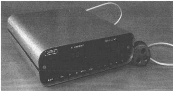
Fig.5 The measurement device with the digit display of UV radiation with the intensity in limits of values 10^{-4} ÷ 2 \cdot 10 mW/m 2 the spectral domains, nm: 280÷400, 320÷400, 320÷360; the dose - 0 ÷ 1.6 \cdot 10^5 J/m 2 . The current supplying – 220 V
