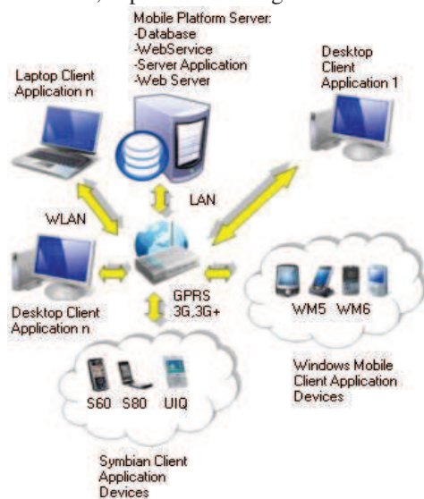
Fig. 1 The hardware and software architecture of the mobile platform
